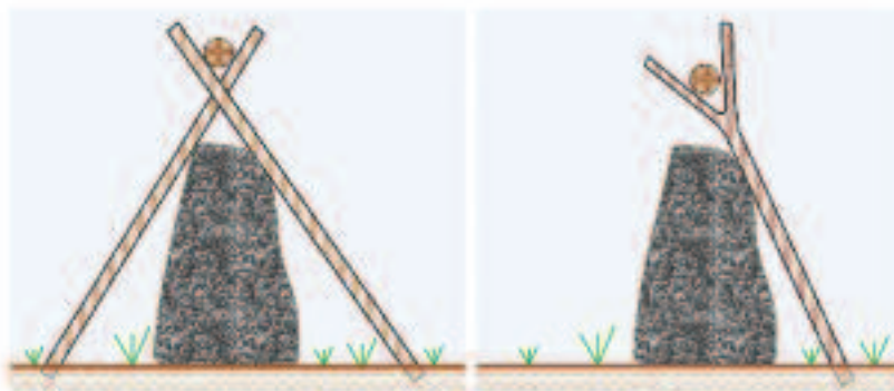
Using dog-legs ( left ) and forks ( right ) to support a log above walls to increase the height of the fence, or to quickly repair a partially fallen wall.
